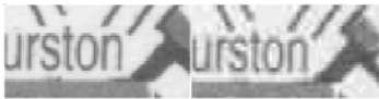
Effects of Lossy Compression on Text: Close-up comparison of a section from a map saved in lossless GIF (left) and lossy JPEG (right).
